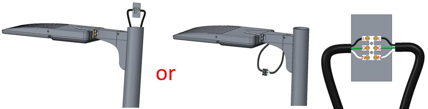
Step5: Mount the bracket cover at the bottom of the bracket.
