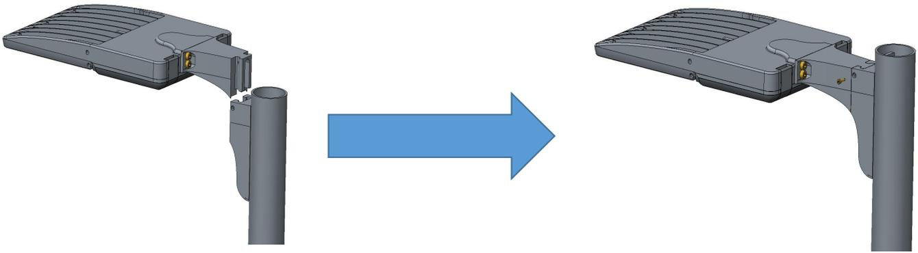
Step4: Wiring, connect the L,N,GND wires on the lamp to the corresponding L,N,GND cables on the pole.
