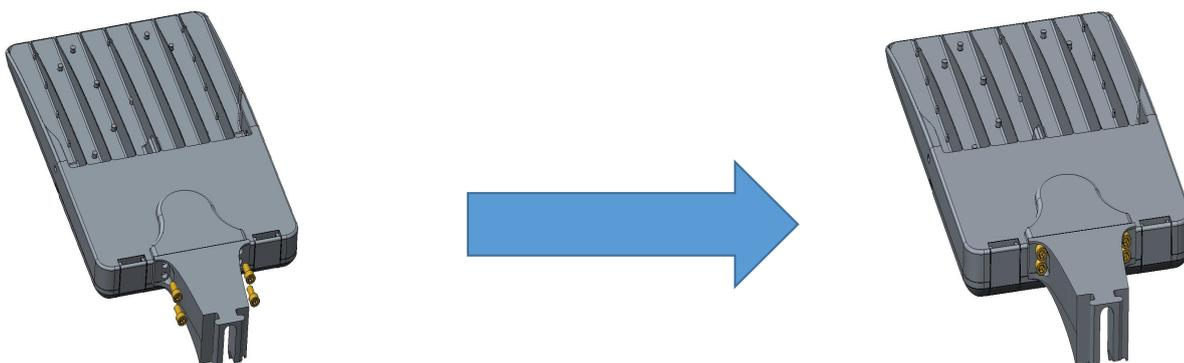
Step2: Mount bracket B on the pole and screw it.
