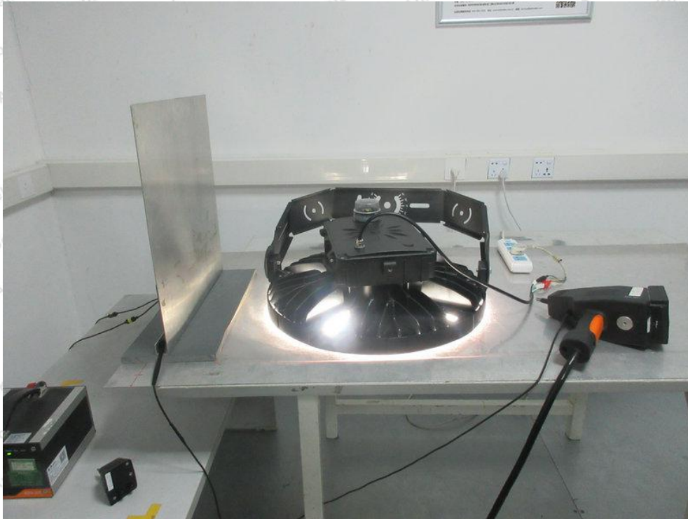
Photo of Electrostatic Discharge Immunity Test
