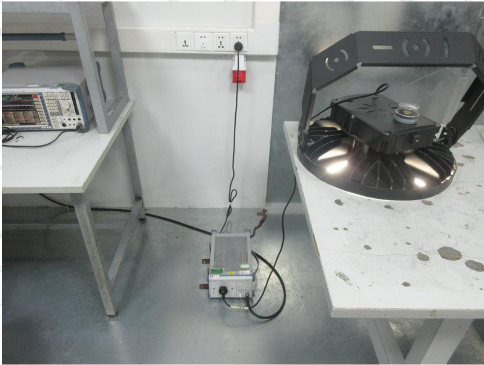
Photo of Power Line Conducted Emission Test
