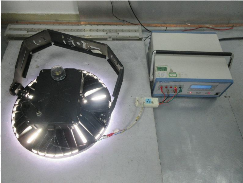
Photo of Electrical Fast Transient/Burst Immunity Test
