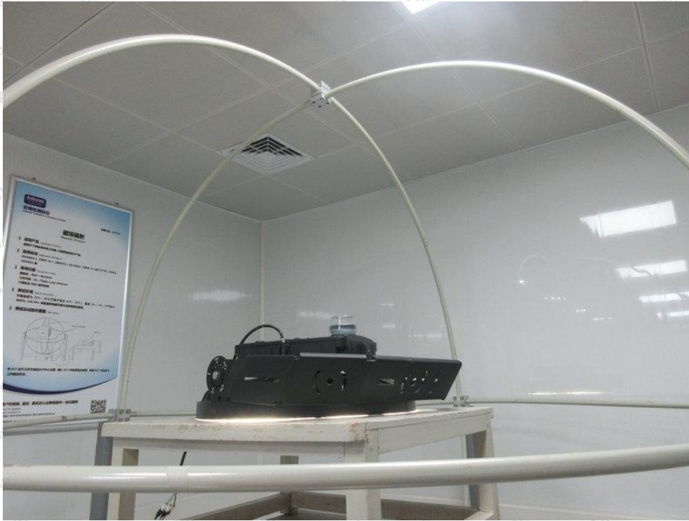
Photo of Magnetic Radiated Emission Test
