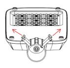
2. Connect the lamp with wire from pole (correspond L, N, GND lines), then according to the arrow direction of the lamp bracket inserted into the lamp pole (can be used on 40-63mm light poles), as shown below.
