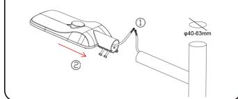
3. Tighten the four screws of the bracket as shown below.
